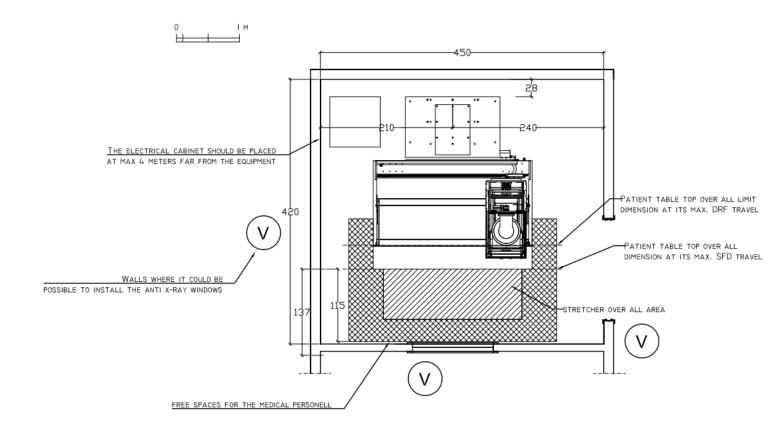
In case of DRF the depth could be reduced from 420 cm to 380 cm
